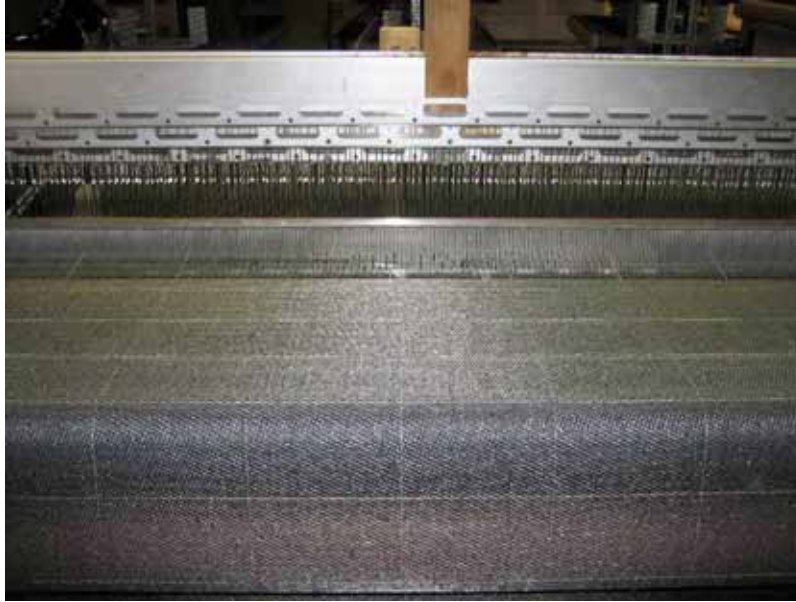
Figure 8: Carbon DiscoTex ® fabric with discontinuous glass tracers rolling off the loom at Pepin Associates, Inc.
